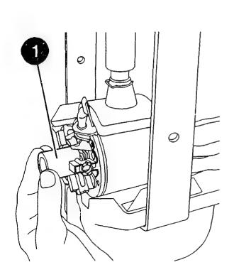
Disassembling overrunning-clutch drive Attach disassembly sleeve (1) to drive shaft such that collar of sleeve is facing upwards. Tap firmly (plastic-headed hammer) on assembly sleeve to knock back stop ring.
